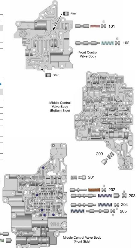
Middle Control Valve Body Descriptions I.D. No. Description 201 Pressure Relief Valve 202 Lockup Control Solenoid Valve 203 3-4 Shift Valve 204 2-3 Shift Valve 205 1-2 Shift Valve Solenoid B-1 Modulator 206 Valve No.1 207 Accumulator Regulator Valve Primary Regulator Valve 208 & Boost Assembly Pressure Relief Valve 209
