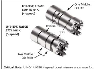
**Critical Note:** U140/141/240 4-speed boost sleeves are shown for reference. These **CANNOT** be interchanged with U151E/F, U250E 5-speed units or line pressure problems will occur.
