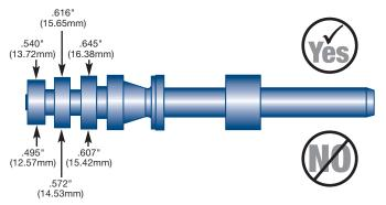
Do NOT use Sonnax valve to replace OEM valve if the valve spool diameters match these bottom measurements:
