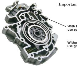
Important: Care must be taken to install the correct pin style or line pressure and pump performance will be affected.
