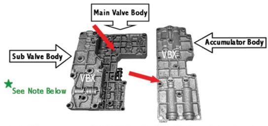
We stock 3 different types of E40D Valve Bodies. Each model varies, depending upon casting numbers located on the Main Valve Body and the Accumulator Body. (Please See RED ARROWS above for location of casting numbers.)
