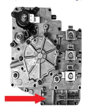
See **RED ARROW** above. Please refer to this area of Valve Body for a Casting Number starting with either XF or YF.
