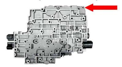
To identify a 4L80E Valve Body from years 1991-1996, look for two small holes on the upper right side of the Valve Body (see **RED ARROW**). The holes do not appear on the Valve Body from for model years 1997 & Up.
