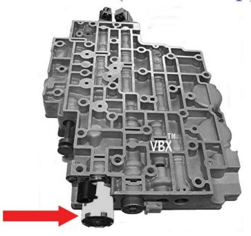
The 2004 & Up version of the 4L80E Valve Body has a late style EPC which can be identified by the silver canister. Please see **RED ARROW** above for location of the EPC.
