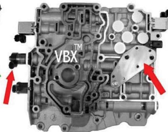
The 4T65E Valve Body for model years 1997 - 2002 has a Holley Type EPC and a larger PSI Manifold. (See **GREEN ARROWS**).
