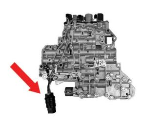
Our RE4F04A and RE4F04B Valve Bodies contain exclusive VB-Xtra updates that prevent open throttle slipping and allow the transmission to shift more efficiently.
