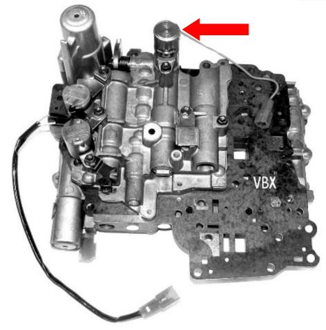
The Toyota A541E Valve Body has a fourth solenoid for lock-up located opposite the filter side of the Valve Body.
