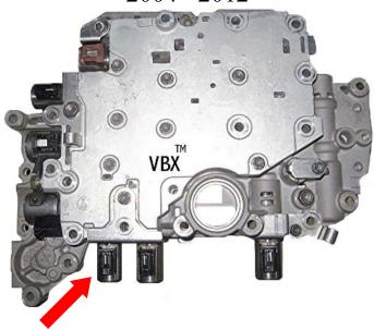
The valve bodies <u>CANNOT</u> be interchanged! The linear solenoids are different in size! The electrical connectors on the linear solenoids are different shapes and the internal harness will not plug into the wrong valve body! See <u>RED ARROWS</u> above.
